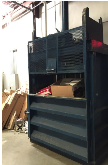
At left, Harnett County Solid Waste has a cardboard baler, which allows the department to bale cardboard for easier disposal.
